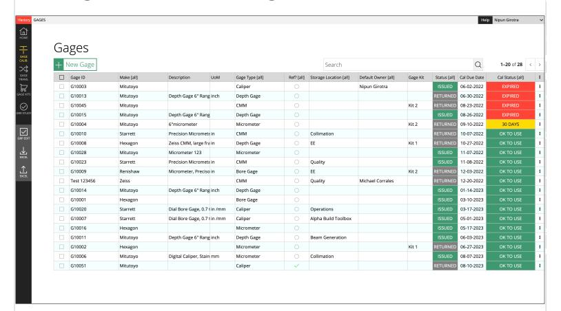
Maintain a list of Gages with calibration due dates. Receive automated notifications for gages due for calibration. Log actual calibration data, and supplier calibration certs.
